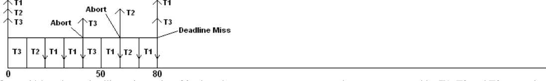
Figure 1(a): \tau_1 has a deadline miss at time 80 when the pr_3 > pr_2 > pr_1 . \tau_1, \tau_2 and \tau_3 are represented by T1, T2 and T3 respectively
