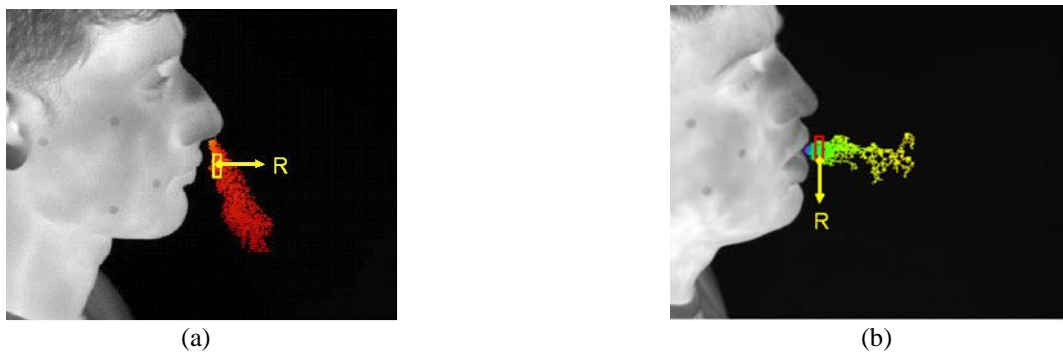
Fig. 2. Respiratory airflow profiles: (a) downward and (b) horizontal.
