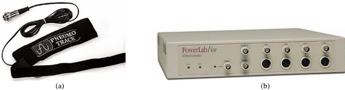
Fig. 11. (a) Piezo-strap transducer. (b) PowerLab Data Acquisition System.
