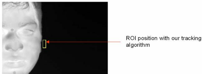
Fig. 19. ROI wrongly positioned when the subject turns his head towards the camera due to the loss of the reference point.
